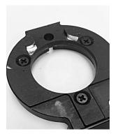
Tape the other lug and file a radius at the corner. Check fit the TRI-LUG to the upper multiple times and continue reprofiling the lugs with the file until it fits.
