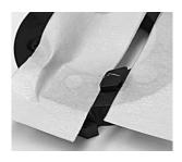
Apply a couple of layers of masking tape to protect the adjoining surfaces.
