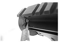
Using an Exacto Knife, scribe a line along the profile of the upper receiver where the lug on the DOLOS interferes with the upper from fitting.
